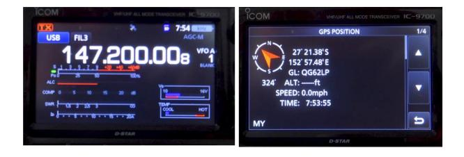
Note the GPS info display is left blank as the GPSD-1 is configured for NMEA RMC message only. That is information about satellites in view is not provided.
