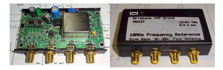
Oven Controlled Crystal Oscillator Operates from a supply of 12 to 28V dc Four SMA outputs. One additional output may be added Calibrated for 10000000.0 Hz Startup 500mA @ 12V dc Settled @12V <250mA; @ 26V <150mA. Sine or square wave > 8 dBm.
