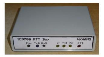
The box is designed to avoid conflict with other applications using the CI-V bus (either 3.5mm or USB). Selecting "transceiver" option in the CI-V menu ensure regular updates of the radio frequency to the box. In this configuration, the box only transmits to the CI-V bus to confirm band when PTT is applied.
