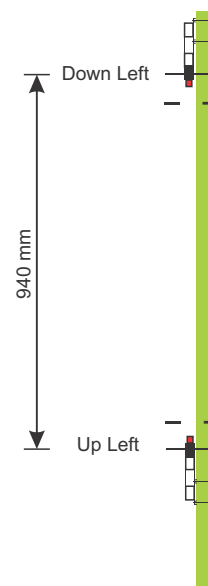
Ver 4. Fiberglass mast 2 different antennas (lower and upper)
